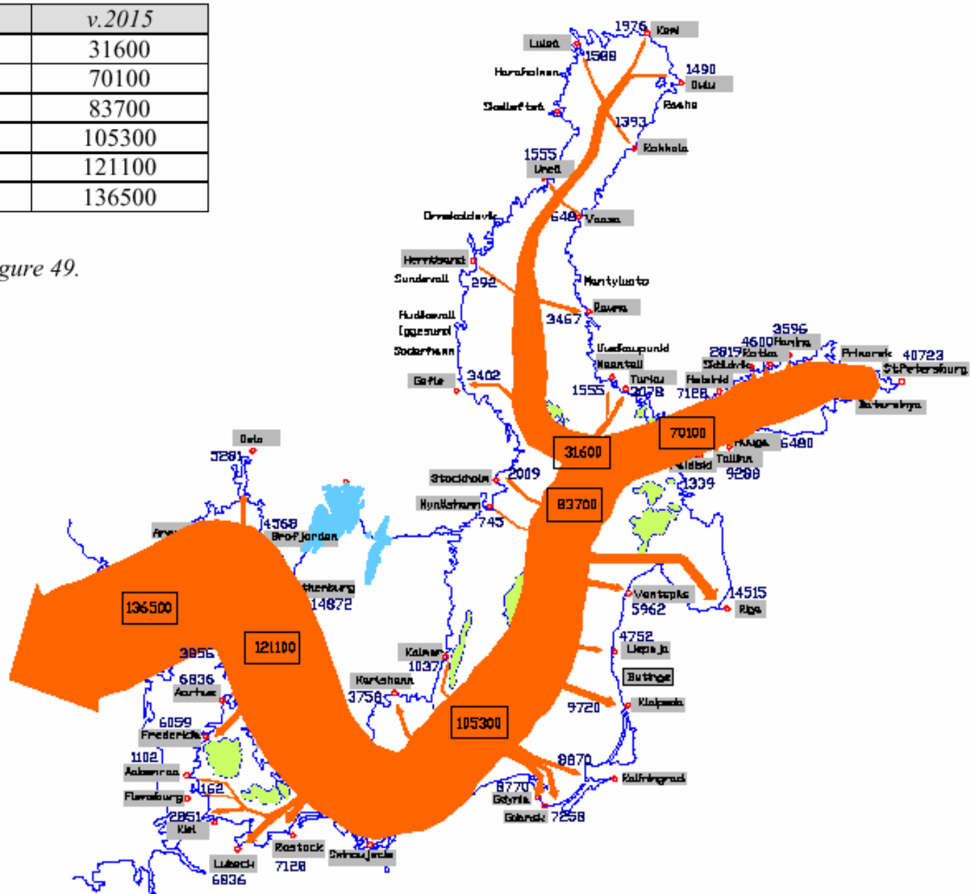
Figure 49. Forecast for the ship movements in 2015. Note: the passenger traffic is excluded.
