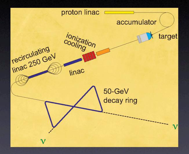
Beam from  $\mu^-$  contains  $\nu_{\mu}$ ,  $\bar{\nu_e}$ , but no  $\bar{\nu}_{\mu}$ ,  $\nu_e$ ,  $\nu_{\tau}$ , or  $\bar{\nu}_{\tau}$ . oscillation studies, scattering on thin targets Beyond the LHC: a Very Large Hadron Collider LHC Discoveries could point to much higher energies
