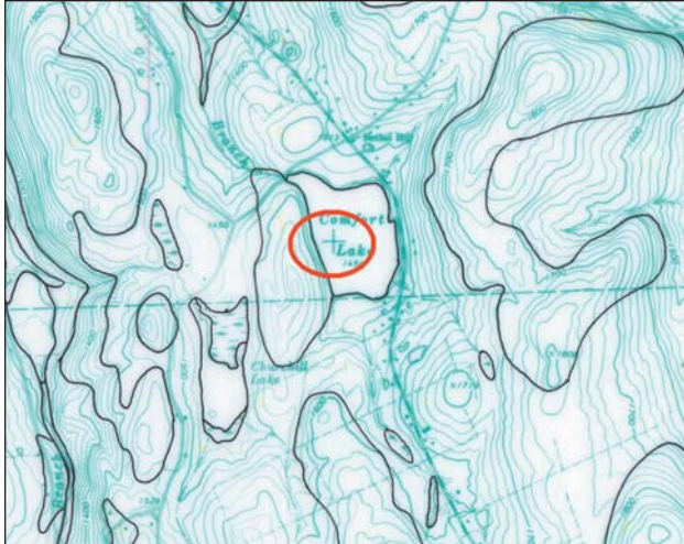
Figure 4. Location control points (tic marks) on the greenline base map are colored green. In order not to lose the control points when the green lines are deleted from the mylar base during scanning, they had to be redrawn in black. Note the location of the green tic mark inside the circle, northwest of the “L” in Comfort Lake. This tic mark had to be changed to black before scanning.
