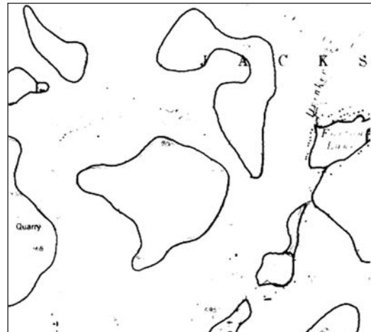
Figure 6. Setting the threshold too low picks up unwanted background lines from the greenline, and “noise” along with the geologic contact lines.
