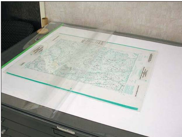
Figure 2. Folded clear acetate sheath for scanning. A sheet of plotter paper is placed behind a greenline or overlay mylar to provide a white background for contrast. This set-up is also good for protecting fragile maps from friction involved in the scanning process.
