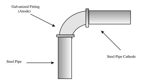
The galvanized elbow will act as an anode to steel and will corrode. <u>Do not install galvanized</u> pipe or fittings in system, if possible.
