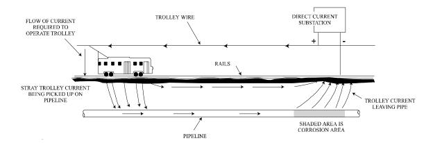
This drawing illustrates an example of stray d.c. current getting onto a pipeline from an outside source. This can cause severe corrosion in the area where the current eventually leaves the pipe. Expert help is needed to correct this type of problem.
