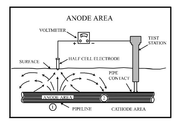
The voltage potential in this example is the difference between points 1 and 2. Therefore, the current flow is from the anodic area (1) of the pipe to the cathodic area (2). The half-cell is an electrode made up of copper immersed in copper-copper sulphate (Cu-CuSO<sub>4</sub>).
