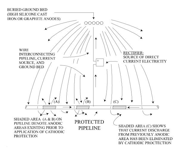
This illustrates how cathodic protection can be achieved by use of a rectifier. Make certain the negative terminal of the rectifier is connected to the pipe. **NOTE**: If the reverse occurs (positive terminal to pipe), the pipe will corrode much faster.
