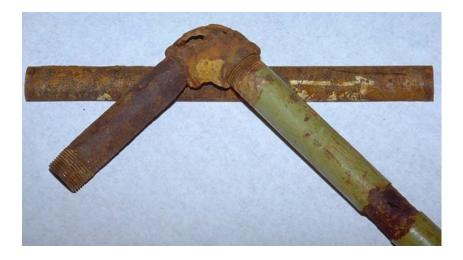
An example of a main which was buried without a coating or wrapping at the service connection. This corrosion problem could have been avoided by properly coating and cathodically protecting the pipe.
