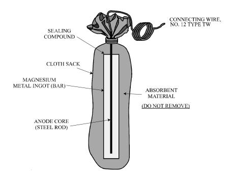
**Sacrificial protection** means the reduction of corrosion of a metal (usually steel in a gas system) in an electrolyte (soil) by galvanically coupling the metal (steel) to a more anodic metal (magnesium or zinc) (see FIGURE III-3). The magnesium or zinc will sacrifice itself (corrode) to retard corrosion in steel the pipe.
