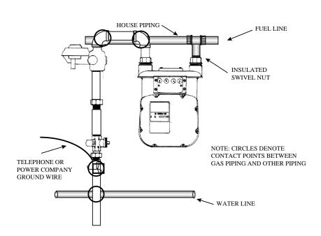
Unshaded piping shows Operators piping from service entry to meter insulator at location shown on sketch above. Shaded areas show house piping, electrical cables, etc.
