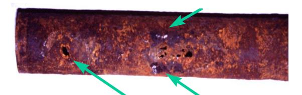
An example of bare steel pipe installed for gas service. Note the deep corrosion pits that have formed. Operators should never install bare steel pipe underground. Operators should use either polyethylene pipe manufactured according to ASTM D2513 or coated steel pipe as new or replacement pipe. If steel pipe is installed, that pipe must be coated and cathodically protected.
