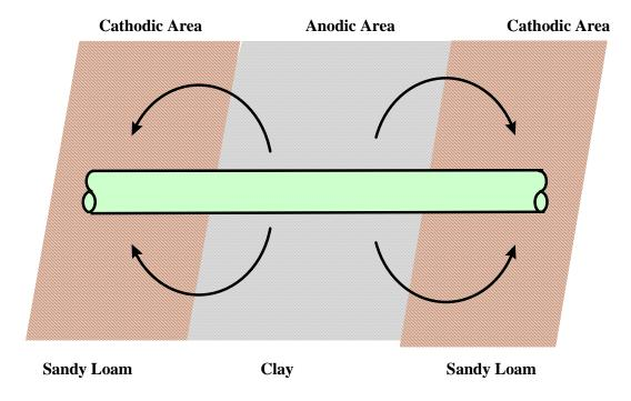
A corrosion cell can be set up when pipe is in contact with dissimilar soils. This problem can be avoided by the installation of a well-coated pipe under cathodic protection.
