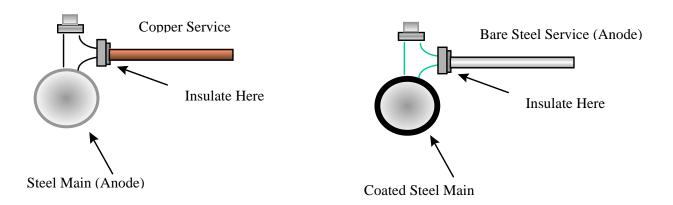
Steel is above copper in the galvanic series in TABLE 1 of this chapter. Therefore, steel will be anodic to the copper service. That means the steel pipe will corrode. The copper service should be electrically isolated from the steel main. Remember, steel and cast iron or ductile iron should not be tied in directly. Steel and cast iron should be electrically isolated. Also, coated steel pipe should be electrically isolated from bare steel pipe.
