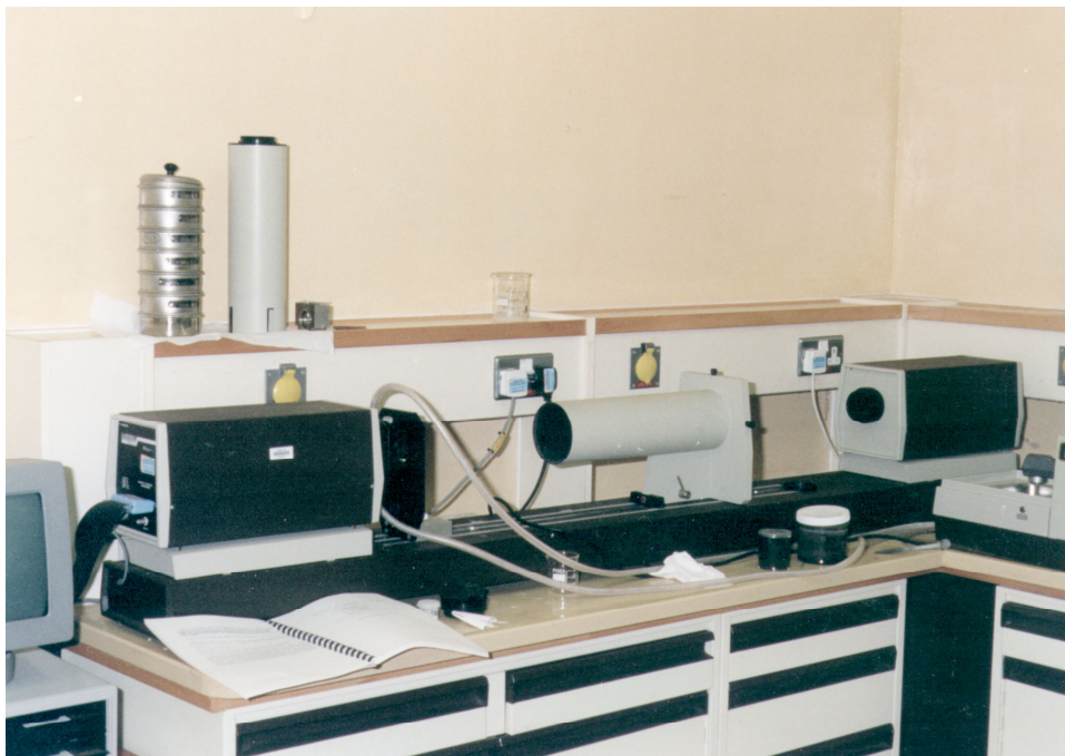
Fig. 2. Photograph of laser light scattering equipment for flow precipitation studies.
