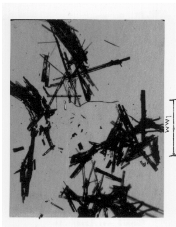
Fig. 17. Microphotograph of sample of crystals from the filtered SX-104 precipitate.
