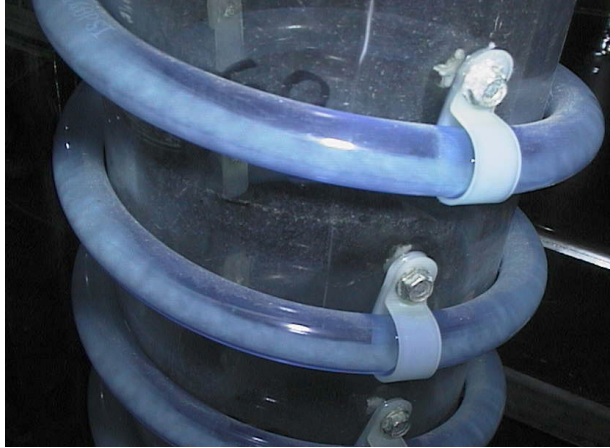
Fig. 4. Clear tubing partially plugged at test section (AN-103 simulant).
