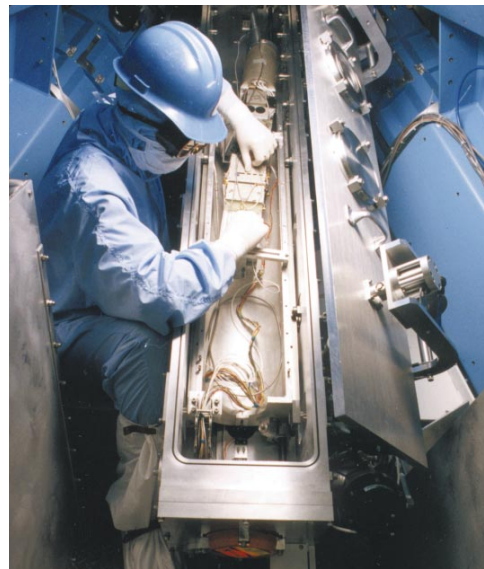
Livermore scientist Ted Perry adjusting a gated x-ray imager on the Omega target chamber. While the National Ignition Facility is being built, teams of Livermore scientists travel to Rochester regularly to do experiments on Omega in support of stockpile stewardship and to advance their understanding of laser target physics.
