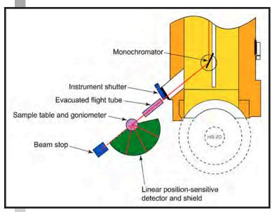
resolved experiments for structural transformations having short time constants. The WAND detector (ORDELA 1410N) is a multianode type (624 anodes and a  $0.2^{\circ}$  pitch) <sup>3</sup>He gas counter specially designed for this instrument. This detector has an intrinsic angular resolution of 0.25° and a maximum counting rate per anode of  $10^5$  counts/s.
