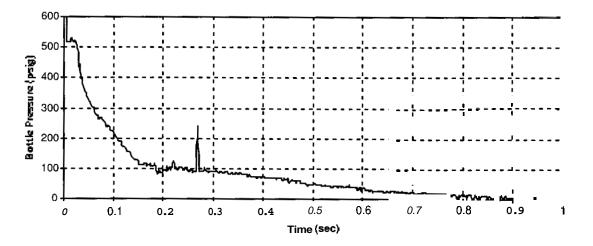
Figure 14. FM200 Blow-down system bottle pressure after -40°C soak.
