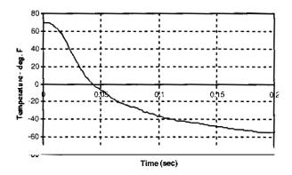
Figure 12. FM200 blow-down system exhaust temperature.
