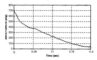
Figure 11. FM200 blow-down system bottle pressure.
