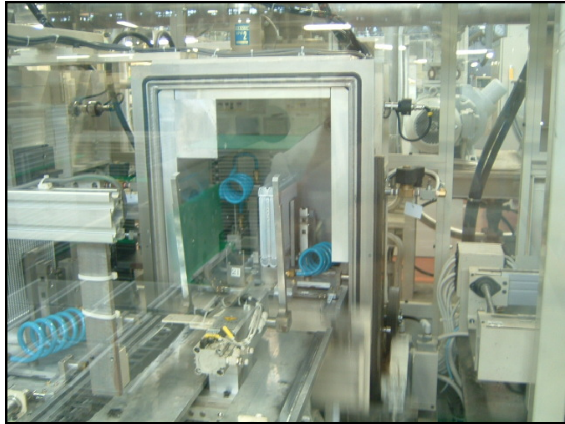
Evaporator leak test
