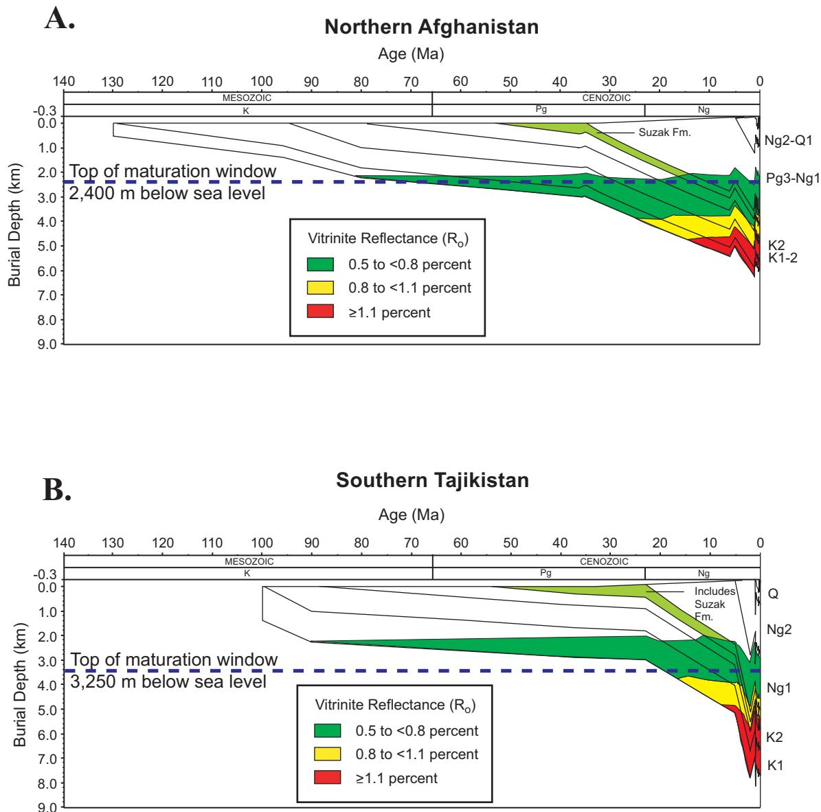
Figure 13. Burial-history curves for the Amu Darya and Afghan-Tajik Basins constructed using the Petromod petroleum-generation model. The thermal window for crude oil generation, catagenesis stage, is where vitrinite reflectance values are between 0.5 or 0.7 and 1.3 percent. Main zone for natural gas and natural gas liquids/condensate generation is where vitrinite reflectance values are between 1.3 and 2.0 percent.
