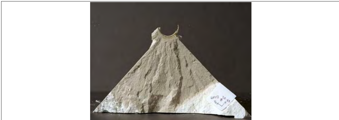
Figure 35. Fracture front splitting observed in a laboratory model test on hydrostone, with a large stress difference between the in-plane and out-of-plane stresses (Van Dam, 1999)
