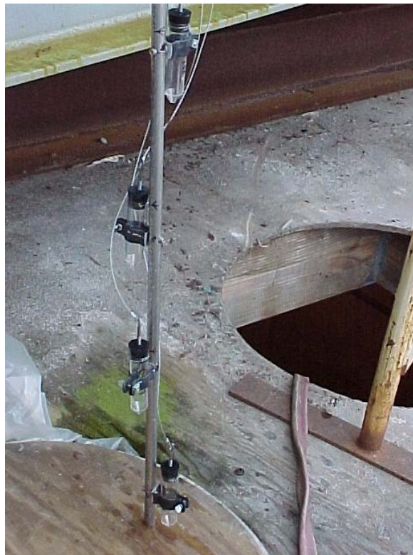
Fig. 30. End of long-pole sampling tool, showing sample collection vials.
