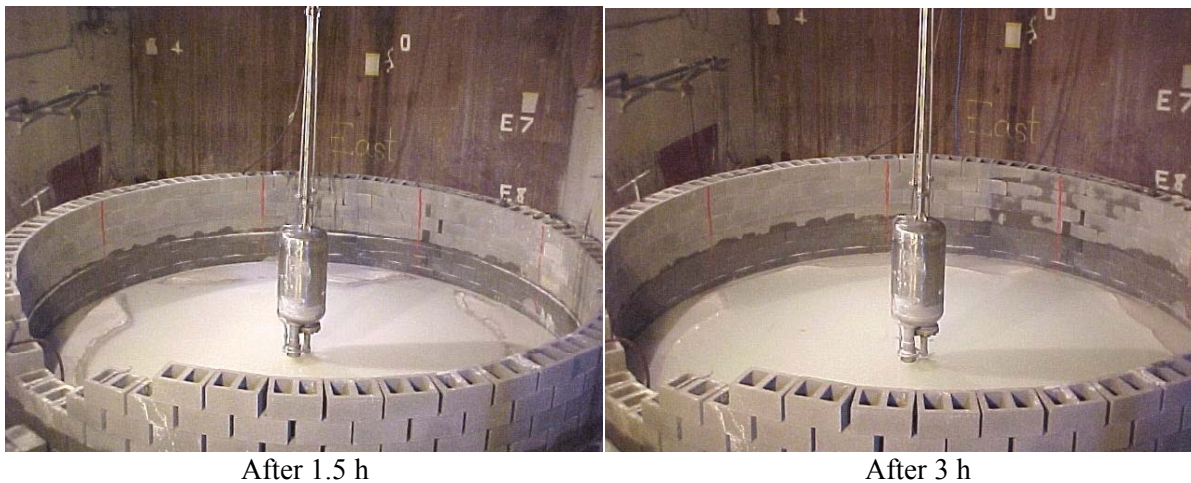
Fig. 29. View of mock-tank after mixing a single in-line clay-sand mound.
