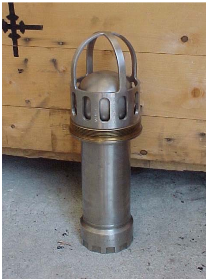
Fig. 10. Check valve assembly before installation in the bottom of the PMP PV.
