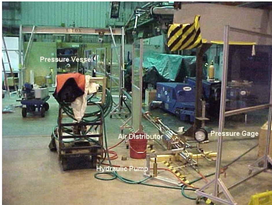
Fig. 5. Russian PMP hydrostatic test setup.
