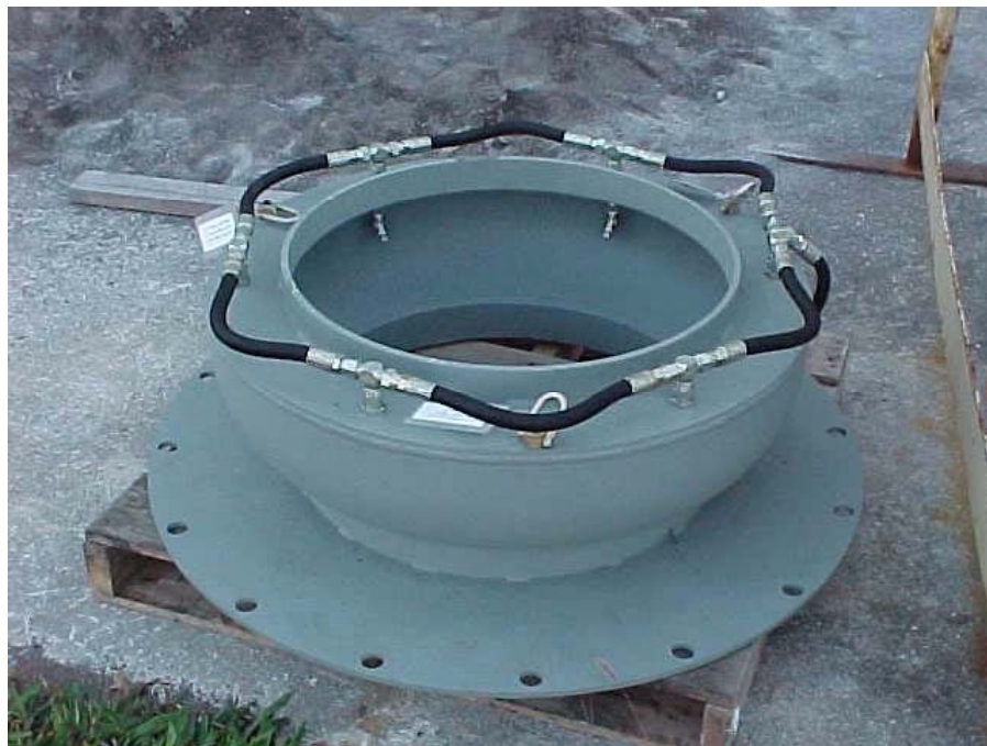
Fig. 8. DSR at the TTCTF prior to installation for cold testing.
