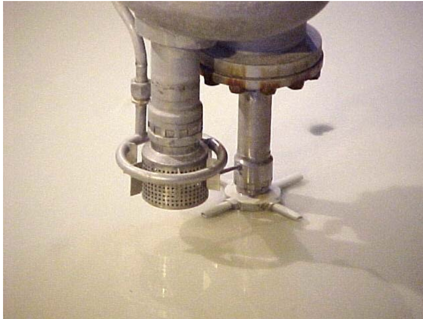
Fig. 17. View of the bottom of PMP showing the orientation of the screened inlet port relative to the discharge nozzles.
