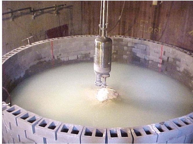
Fig. 28. View of clay-sand mound before mixing and filling of mock-tank.
