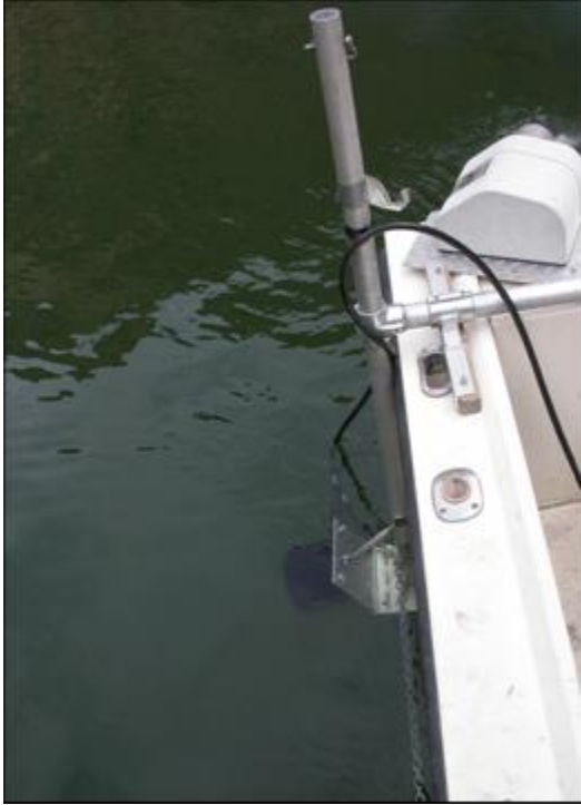
Figure 3-3. Transducer Mounts for Columbia River Surveys
