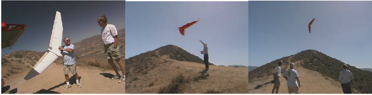
Figure 16. Sandia test glider, the “DS Beast” is used to collect the first airborne data during a dynamic soaring flight at Parker Mountain, California on Nov. 16, 1999. Left: Plane Builder Pat Bowman holding glider with P.I. Center: Pilot Joe Wurts launching into wind. Right: Glider executes upwind dynamic soaring run on leeward side of ridge (Photo: Dave Reese).
