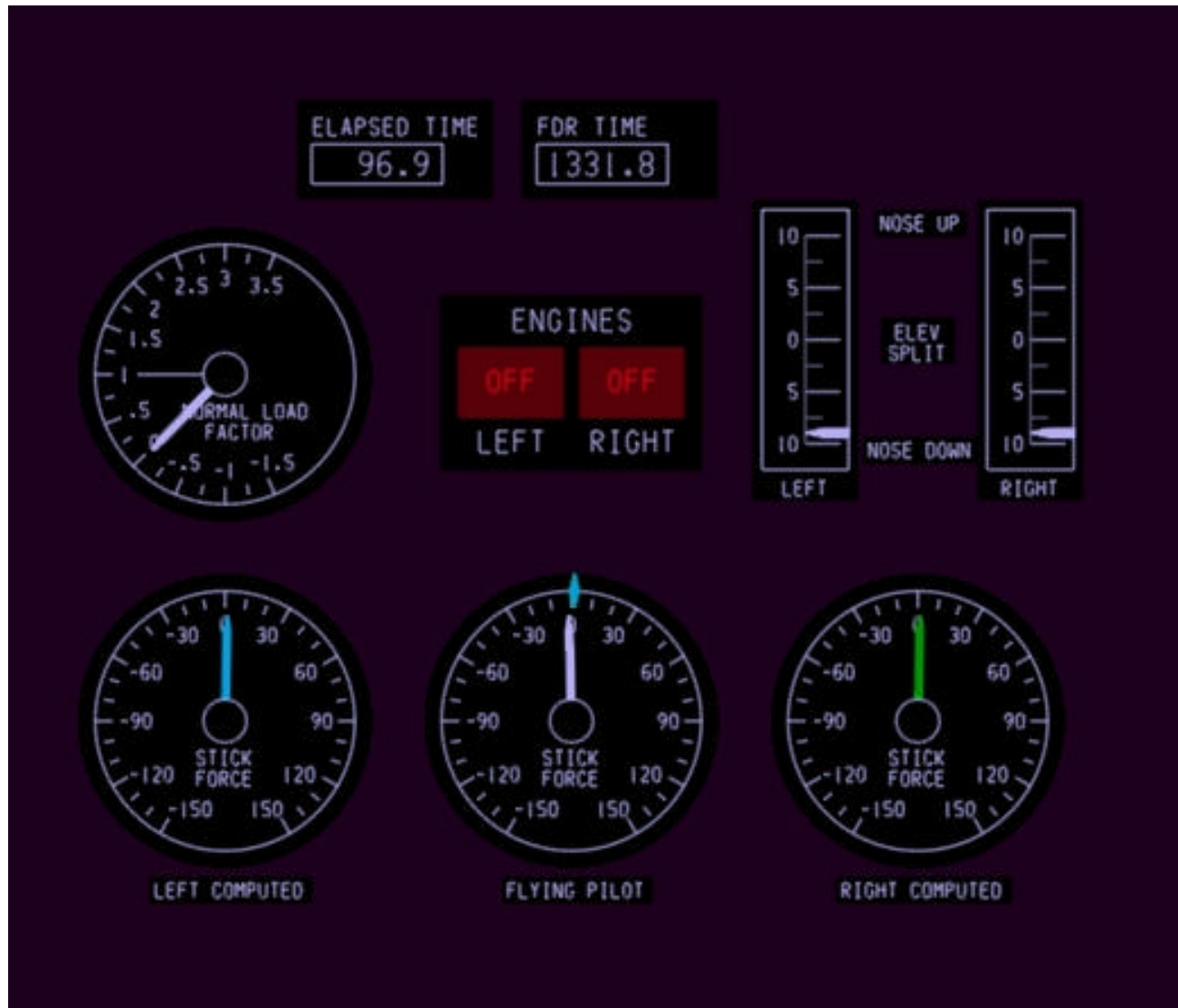
Figure 14. Visual system instrument display for March 2000 E-CAB simulations.
