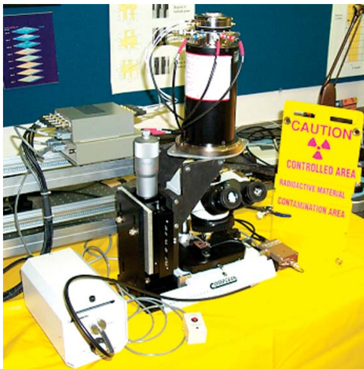
Figure 2. Prototype of alpha particle table IPEM, with the "Mepsicon" position sensitive detector (PSD) on top of the microscope.
