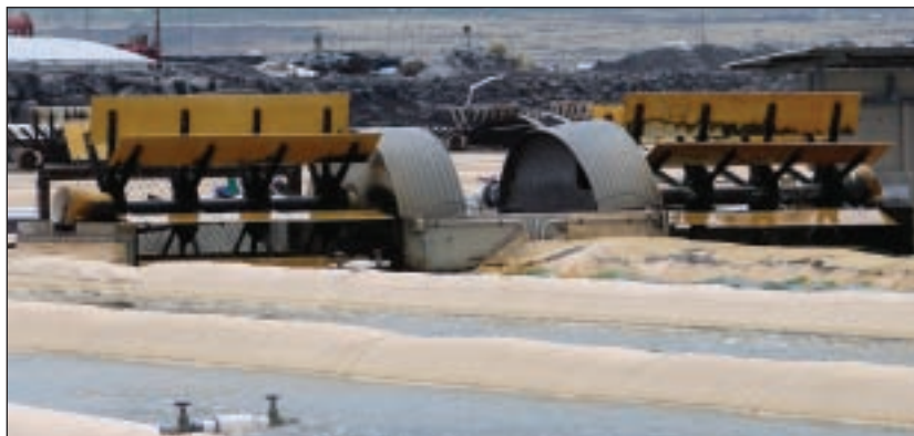
Commercial aquaculture operations use paddlewheel technology in land-based systems to farm microalgae.
