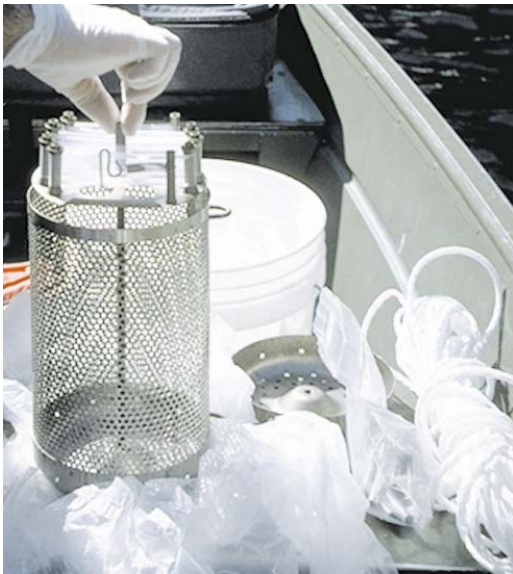
Semipermeable membrane sampling device, Upper Angora Lake, Calif., July 1998. Photograph by K.J. Hill, Tahoe Regional Planning Agency.
