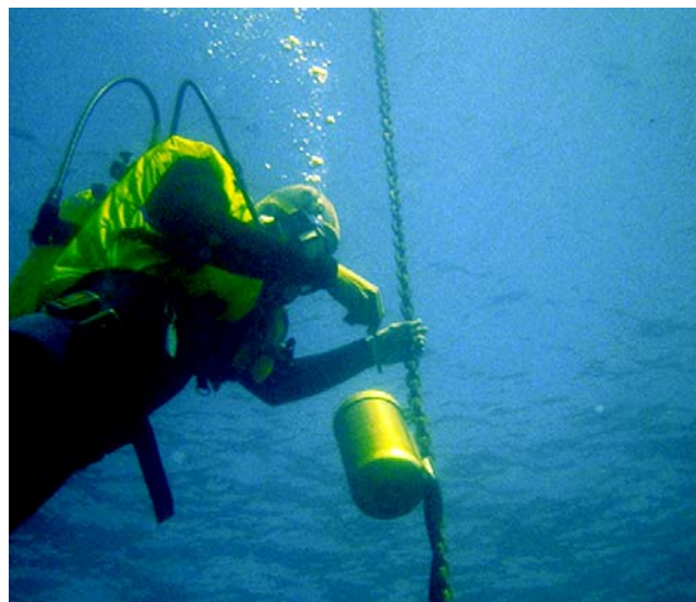
Diver retrieving semipermeable membrane device from Lake Tahoe, near Glenbrook, Nev. Photograph by R.J. Hoffman, U.S. Geological Survey, August 1998.
