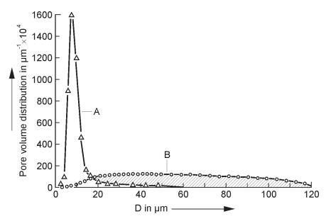
**Figure 3.2.** Comparison of pore volume size distributions for Clear Creek sandstone: curve (A) form mercury porosity; curve (B) from photomicrography (sphere model) (Dullien 1975).
