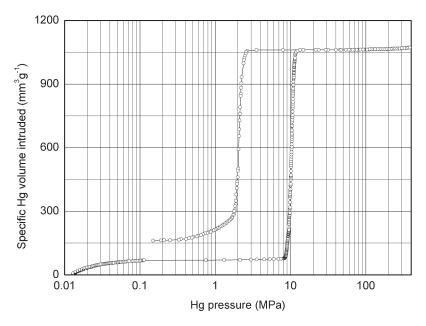
**Figure 6.3.** Intrusion/extrusion curve (volume vs. pressure curve) of a porous glass.
