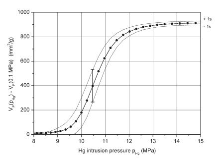
**Figure A.2.4.2.** Certified mercury intrusion curve for CRM BAM-PM-122 with uncertainty intervals in the range between 8 MPa and 15 MPa (linear pressure axis).
