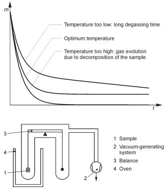
Figure 4.3a. Thermogravimetric control of degassing.
