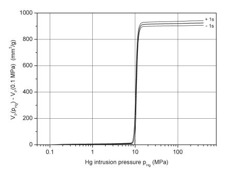
*Figure A2.4.1.* Certified mercury intrusion curve for CRM BAM-PM-122 with uncertainty intervals (logarithmic pressure axis).
