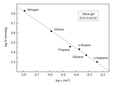
Figure 2.2. Determination of the fractal dimension frm the monolayer adsorption capacity for different test molecules (Noack).
