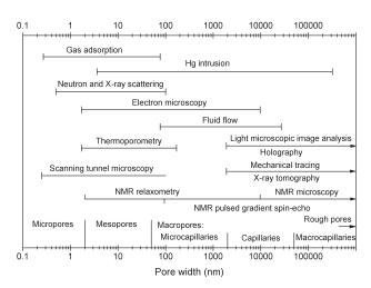
*Figure 3.1.* Measuring ranges of methods for pore size determination (after Meyer 1997)
