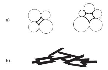
**Figure 1.1.** Pores in different aggregates (Gregg 1982): a) spherical particles; b) plate like particles.
