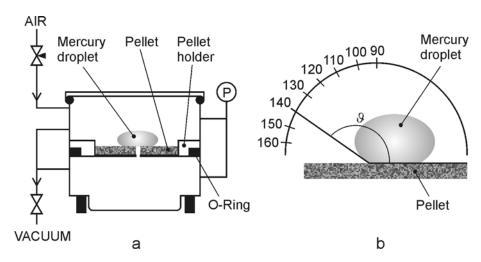
*Figure 6.2. Schematic representation of the (a) advancing angle and (b) static angle method for determination of the contact angle (Groen 2002).*
