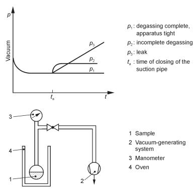
Figure 4.3b. Pressure control of degassing.
