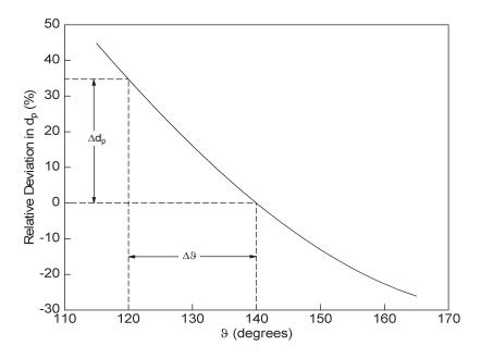
**Figure 6.1.** Relative deviation in the calculated pore diameter  $d_p$  as a function of the mercury contact angle  $\vartheta$  (reference value 140°).
