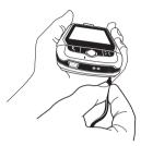
The orange charge indicator light will go on and a lightning bolt icon will appear over the battery icon in the title bar, indicating the charger is connected and the battery is charging. Note that if your device has discharged completely, it may take up to 15 minutes before you see any indication of charging on the screen.
