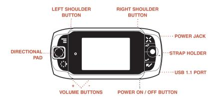
**DIRECTIONAL PAD (D-Pad)** Press up/down/left/right to scroll or move within text fields, and navigate in games. The D-Pad "rocks" in four different directions and generally mirrors the behavior of the trackball.
