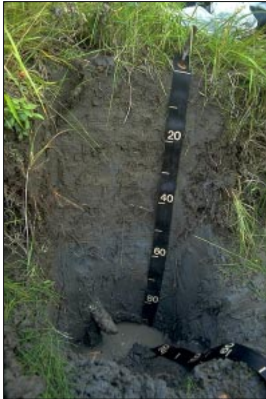
Upper: Swedna, very poorly drained, soils on a low flood plain adjacent to the channel. Bluish coloration below 50 cm (20 inches) is the result of continuous saturation and hydromorphism.
