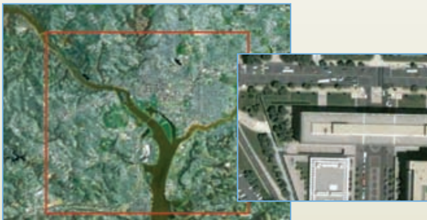
The Sonoma surveillance system offers the resolution shown on the right, covering the area outlined in red, from a single airplane-mounted camera. The satellite image is of Washington D.C.
