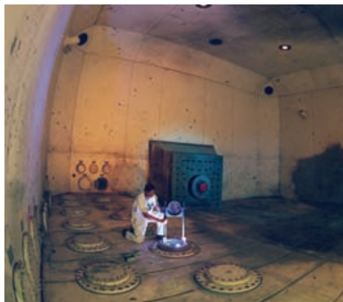
Inside Site 300's Contained Firing Facility, John Given sets up equipment for a "shot" as part of large-scale hydrodynamics testing. These tests are essential for verifying the safety and reliability of the nuclear stockpile.
