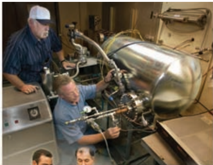
Vern Switzer and Tim Ross (top) work on a new hydrogen fuel tank for a Toyota Prius, shown below with (from left) Gene Berry, Francisco Espinosa-Loza, and Salvador Aceves.
