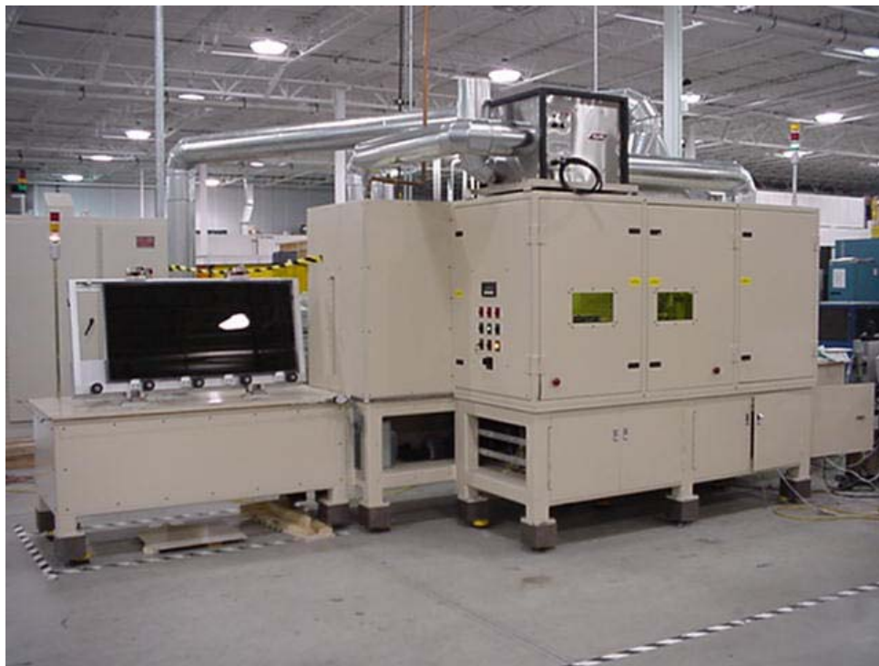
Figure 13. The laser scribing system - the unloading station and system side view
