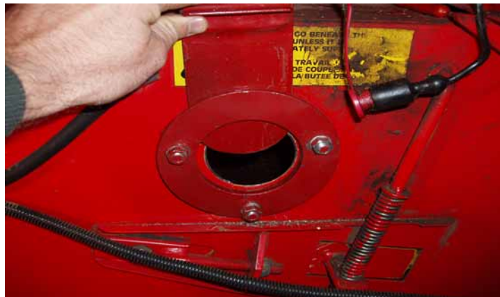
Installed Port Hole
