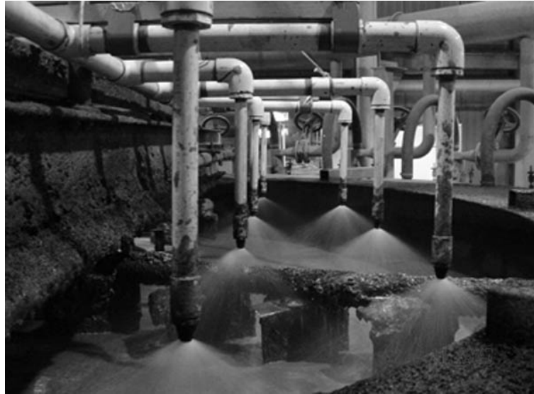
Fig. 2. The GSC flotation cell was fitted with a bank of 14 nozzles for delivery of the surfactant spray onto the surface of the aerated pulp.
