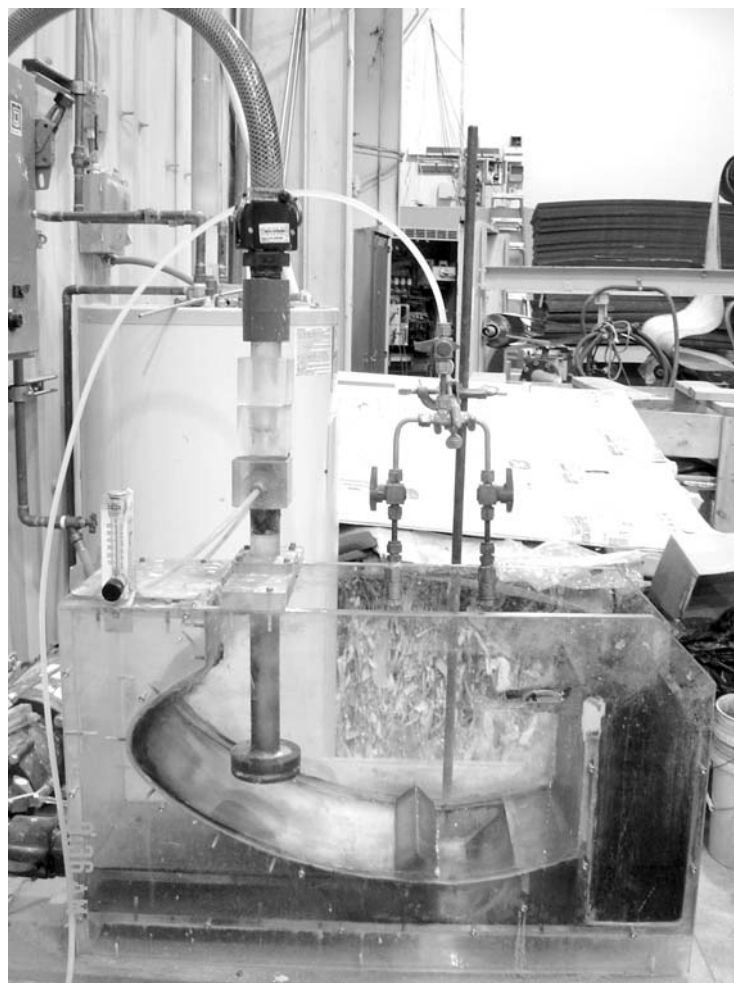
Figure. 2-1. Side view of the E-18 flotation cell equipped with dual nozzles for surfactant spray delivery.
