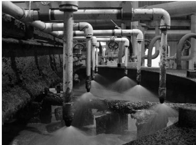
Fig. 4-2. The GSC flotation cell was fitted with a bank of 14 nozzles for delivery of the surfactant spray onto the surface of the aerated pulp.
