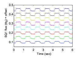
Fig. 3. Plot showing multiplexed optical response of 8 pixels to chopped narrowband 450  $\mu$ m wavelength illumination. The incident optical power on each pixel is 1.8 fW. Plots are offset for clarity.
