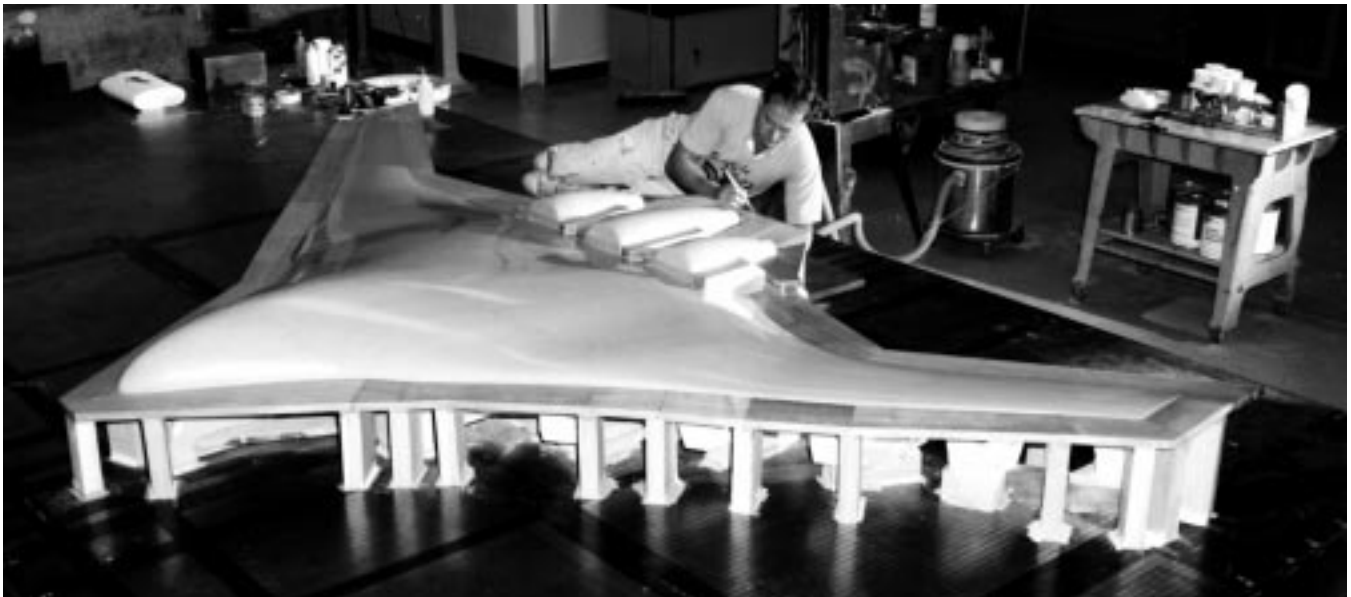
A technician works on the 11-foot wide BWB wind tunnel test model.
