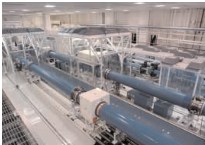
Z-BEAMLET FACILITY'S high bay interior. Rolling clean rooms are in place on each side of beam line. (Photo by Walt Dickenman)
