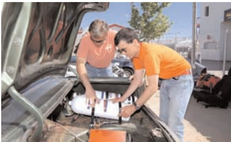
TANK JOB — Mark Grubelich (right) and a friend install nitrous oxide tanks in the trunk of the 1969 Plymouth Valiant, which has been re-engineered and upgraded several times over the last decade.
