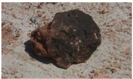
Figure 28. Low Order Detonation Residue on Soil Aggregate
