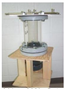
Figure 5. Laboratory Soil Column Test Apparatus.
