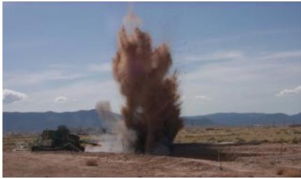
Figure 29. Low Order Detonation (1/3 bag propellant)
