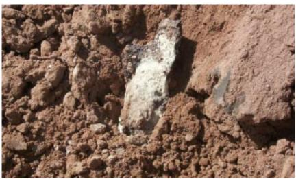
Figure 30. Low Order Detonation Debris (1/3 bag propellant)
