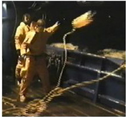
Figure 5: Launch pot and throw out line and buoys
