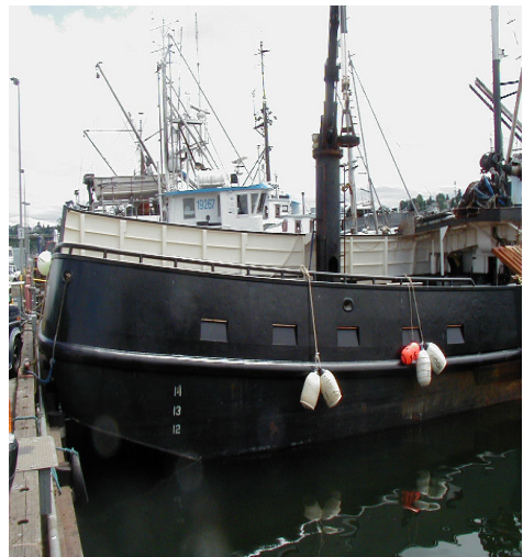
Figure 5: Boat with raised bulwark on port side and raised pipe rail on starboard side
