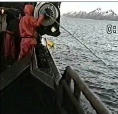
Figure 6: Retrieve buoys, connect line to power pot, bring in pot
