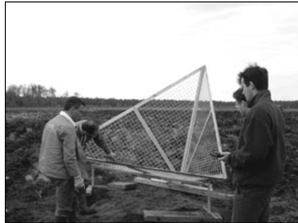
Figure 2: Map of the experiment zone (left) and picture of a P-band reflector (right).
