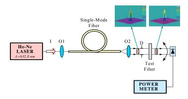
Fig 2. Experimental set-up used to measure the spatial power distribution of the light scattered from the Fog filters.
