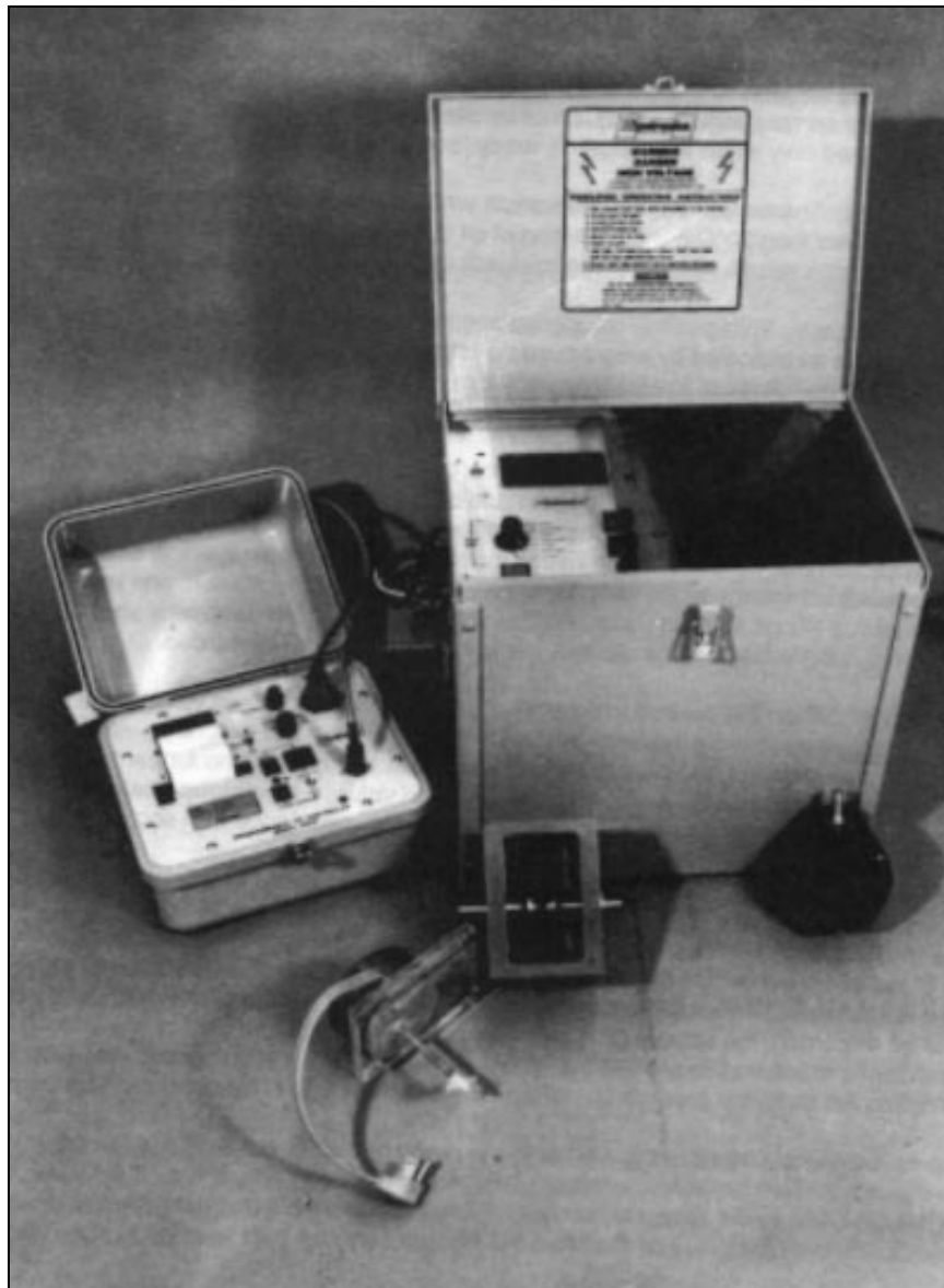
Figure B.1 A Hipotronics Dielectric Test Setup
