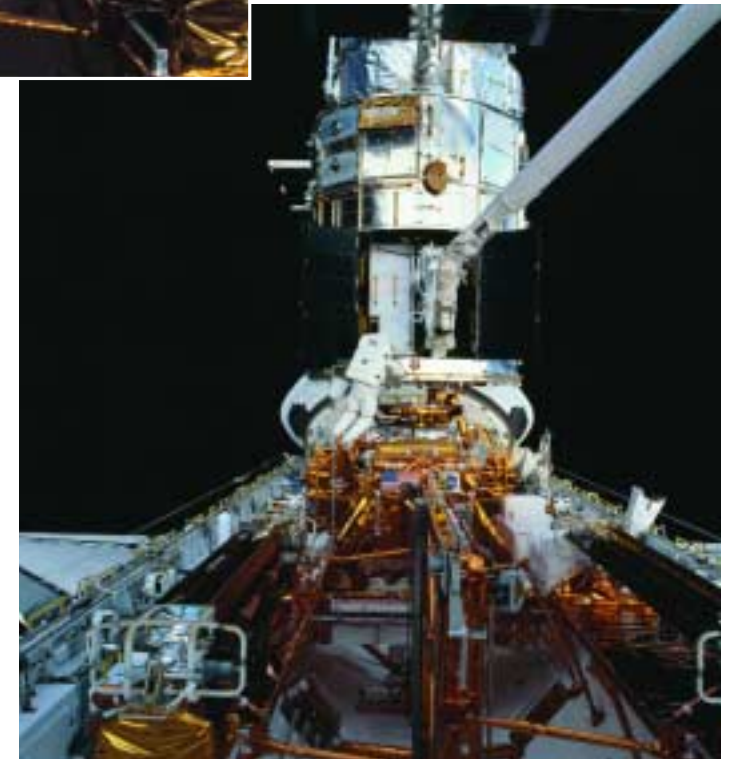
Astronauts James H. Newman, on Columbia's remote manipulator system robotic arm, and Michael J. Massimino participate in the Advanced Camera for Surveys science instrument upgrade during the STS-109 HST servicing mission.
