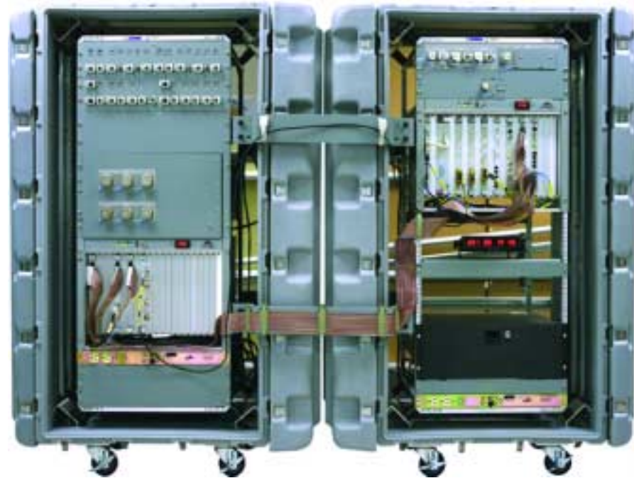
Using the Orbiter-in-a-Box with a Cargo PC SM allows customers to test their payloads with actual shuttle flight software at their own facilities.
