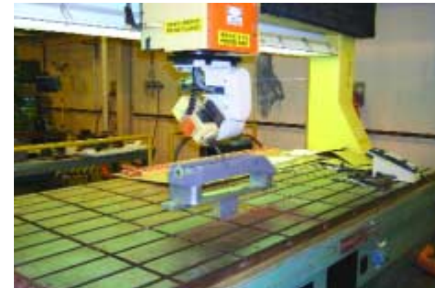
Utilizing existing equipment, Process teams have saved time and cut costs by automating super-light ablator trimming operations.
