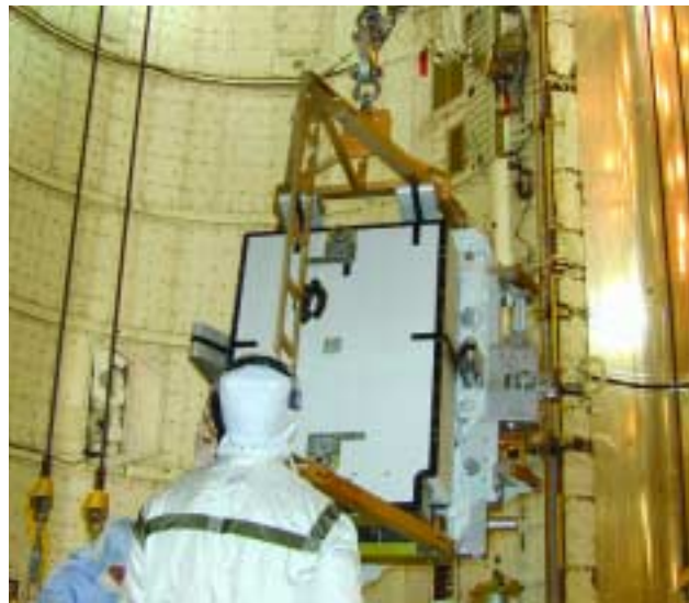
ORUs like the DCSU (shown here being installed in the cargo bay) require quick delivery by the SSP.
