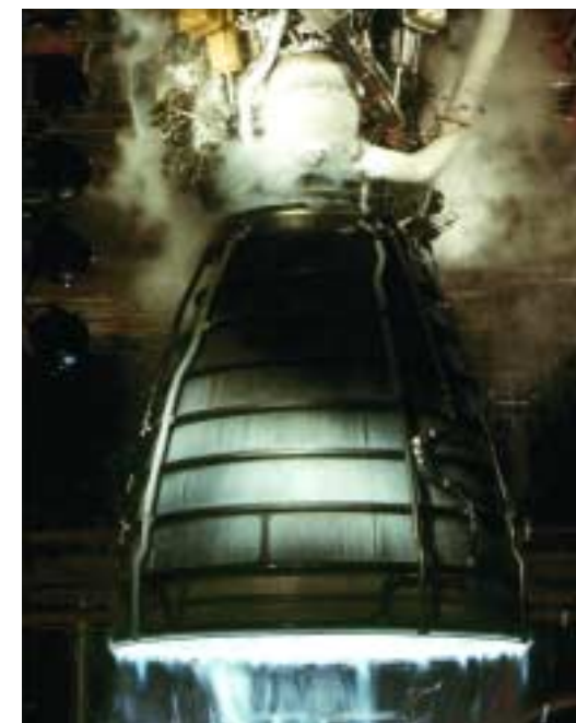
Engines are tested for flight acceptability at Stennis Space Center in Bay St. Louis, Mississippi.
