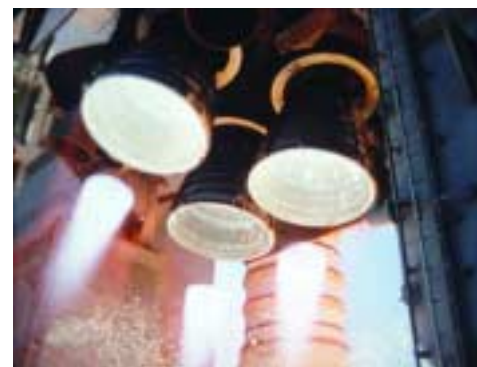
Each SSME produces approximately 500,000 pounds of thrust and runs until the shuttle reaches orbit at 8.5 minutes.
