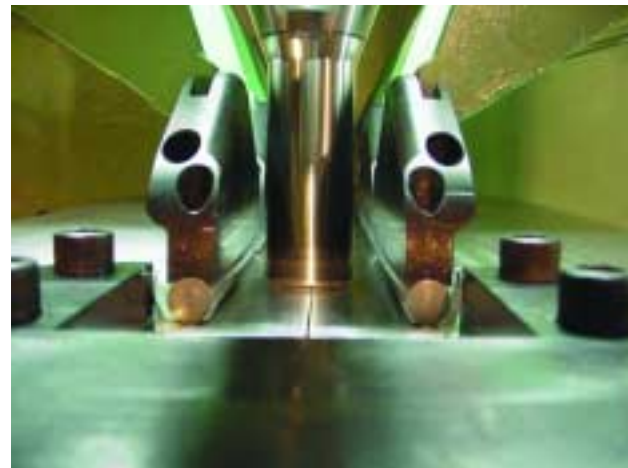
Friction stir weld in process on training unit
