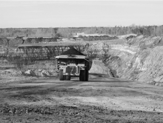
Figure 4. Loaded haul truck coming up pit ramp constructed of ash.
