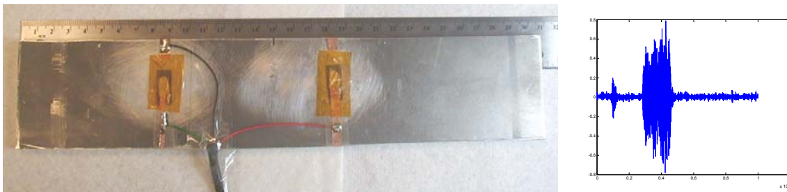
Figure 3.21. Beam with a fatigue crack monitored by two single node neurons. The raw AE signal is shown. In larger structures, the neurons will be continuous fibers.
