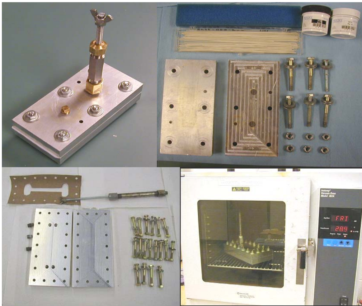
Figure 3.5. Mold for casting AFCS showing original and updated design and curing in an oven.
