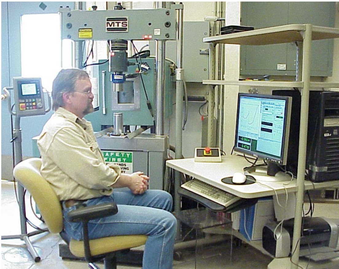
Figure 4. A uniaxial compression test set-up consisting of a 0.1 MN load-frame and environmental chamber for temperature control.
