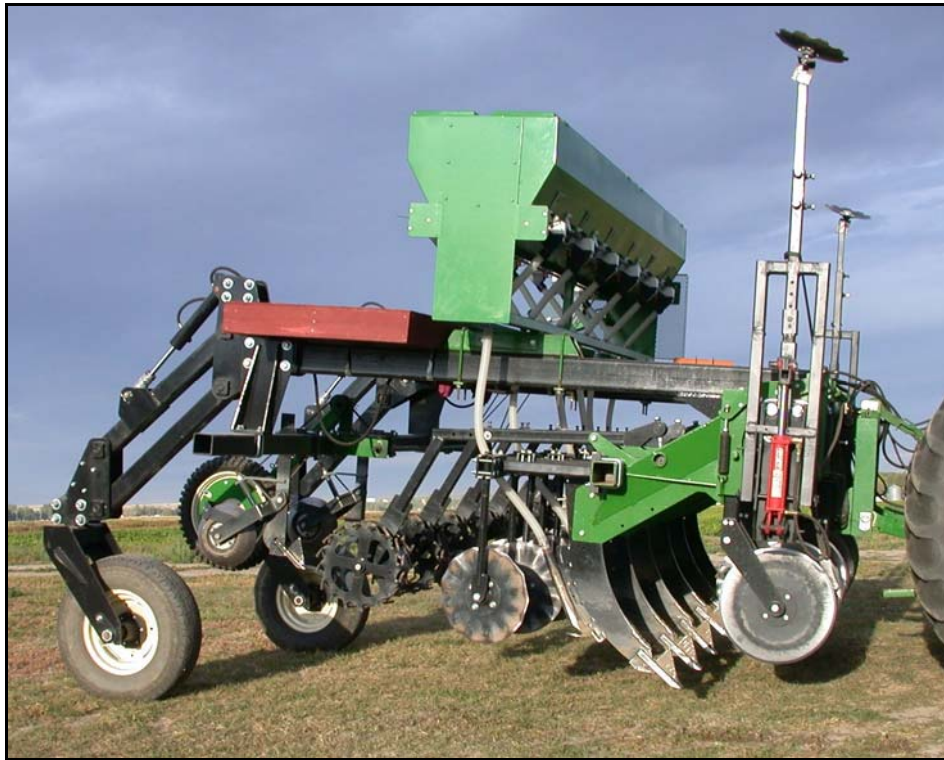
Figure 1. Picture of the custom-built strip tiller showing the progression of disks, rippers and packer wheels.
