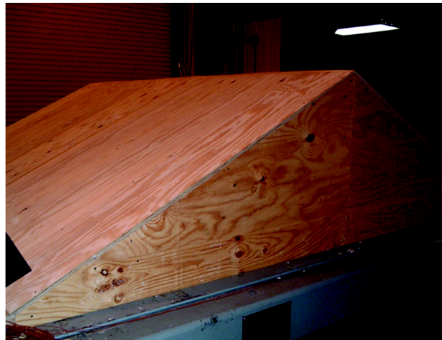
Figure 2 Complete attic module without roofing felt.
