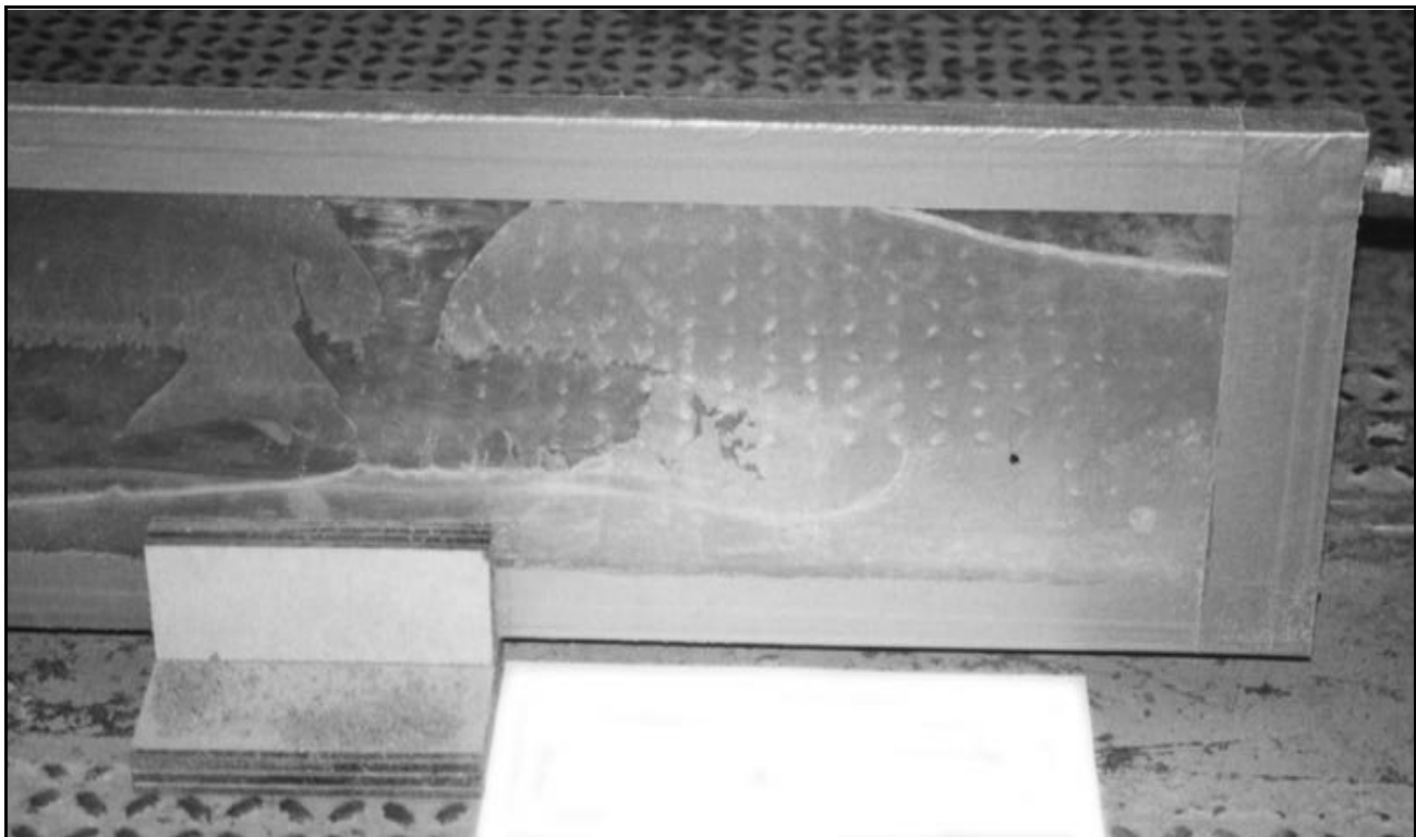
Figure 5 — 1/4" Water Filled Rock Module
