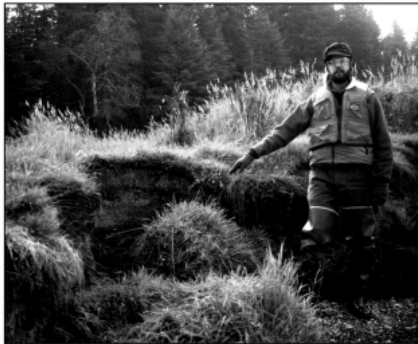
Figure 25. Bank erosion at Skilak Lake study site. Note large pieces of cohesive material that have fallen from the bank.
