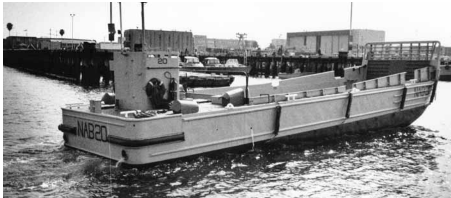
A SANDIA CONTRIBUTION to Operation Desert Storm included development of remote-control landing equipment to assist in mine-clearing and beach-assault operations. Though not actually used in the conflict, the technology was successfully demonstrated on a Navy vessel in San Diego Bay.
