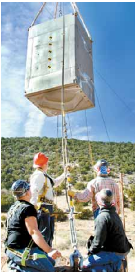
GINGERLY, BOYS, GINGERLY — Team members verrrry carefully help guide a TRUPACT test unit into position for a 30-foot test drop.
