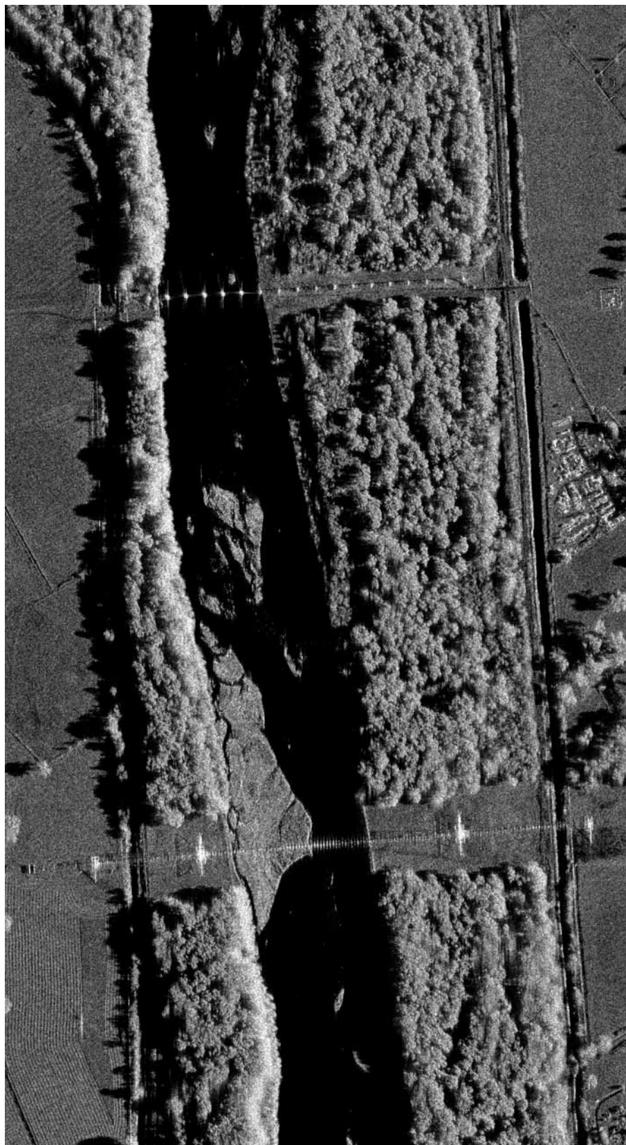
SANDIA’S SYNTHETIC APERTURE RADAR has become a must-have tool for the nation’s military. The photo above, of a small section of the Rio Grande Valley, only begins to suggest the capabilities of this technology, which can image terrain through cloud cover, at night, and in real-time. Sandia continues to refine the technology to meet 21st-century national security threats.
