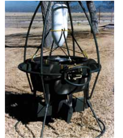
SANDIA'S Airborne Remotely Operated Device (AROD) was developed for use by the US Marine Corps in battlefield surveillance.
