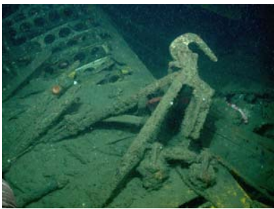
Figure 32. Submerged view of the sky-hook located at the center of the Curtiss Sparrowhawk F9C-2 biplane. The pilot during flight would position the aircraft below the USS Macon's hanger where a trapeze was lowered and the pilot would position the hook onto the trapeze. Sparrowhawk pilots were nicknamed the "men on the flying trapeze". Photo: NOAA/MBARI 2006
