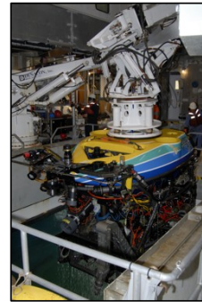
The ROV Tiberon is a remotely operated vehicle used to explore the midwater and deep sea habitats in the Monterey Bay region. Photo: R. Schwemmer, NOAA
