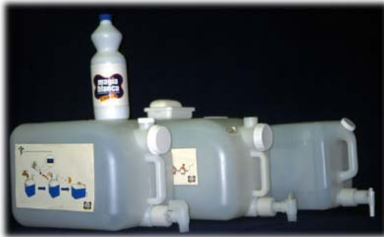
FIGURE 1. The vessel system. Left to right: a five-gallon plastic vessel with a narrow 6-cm mouth and durable faucet for water purification and storage, an identical vessel with detachable soap dish mounted on top, a 2.5 gallon vessel with a 1.5-cm mouth and faucet for storing and dispensing beverages, chlorine, and soap. Pictorial instructions are affixed to the vessel walls.
