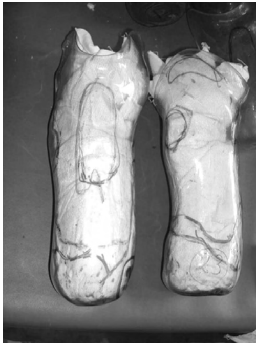
Figure 5. Failed socket (too wide with the result that the weight-bearing area was 2 cm 2 too large and the stump sunk in the socket; check socket right, trial socket left).
