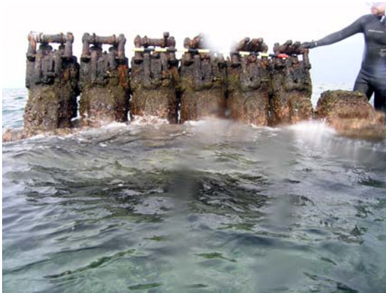
Figures F and G: Imperial Atlas engine on reef crest. Engine skylight and stack/ventilator component in lagoon.
