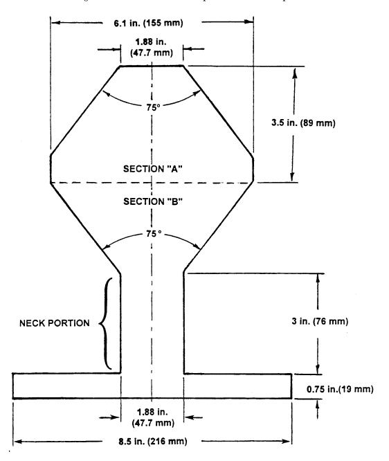
Figure 2 to Part 1213—Test Template for Neck Entrapment
