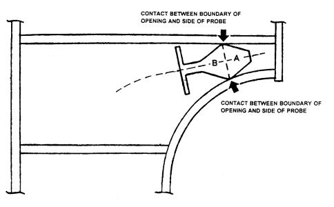
Fig. 3 – Motion of Test Probe Arrested by Simultaneous Contact With Both Sides of "A" Section of Probe and Boundaries of Opening
