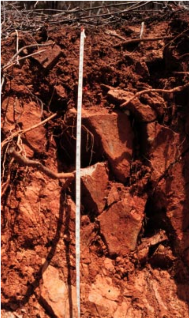
Figure 20. —Profile of Annaberg gravelly loam, in an area of Annaberg-Maho Bay complex, 40 to 60 percent slopes, extremely stony. These shallow, well drained, skeletal soils are on summits and side slopes of volcanic hills and mountains throughout the United States Virgin Islands.
