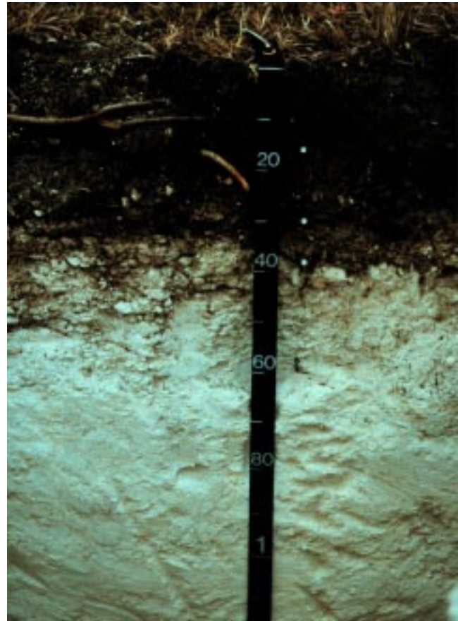
Figure 24.—Profile of Sion clay, 2 to 5 percent slopes, rarely flooded. These very deep, well drained soils are on side slopes and valley floors of calcareous marine deposits on St. Croix Island.
