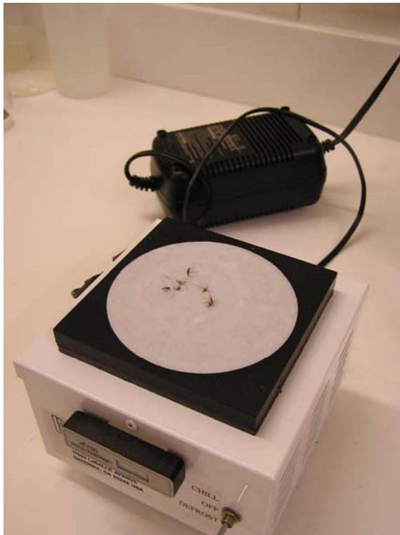
Figure 3.8.2. A small Peltier cold table on which damp filter paper is placed to conduct cold and prevent mosquitoes from sticking to the condensation.
