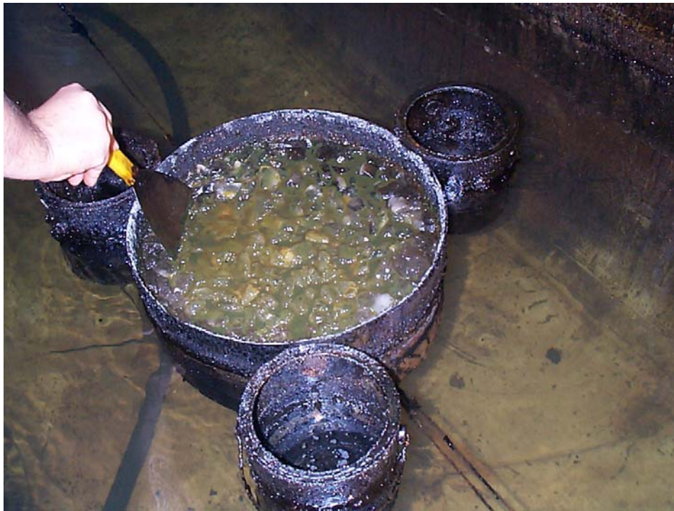
Figure 3-8: Spreading Northstar out evenly on ice surface for minimum ignitable thickness test.
