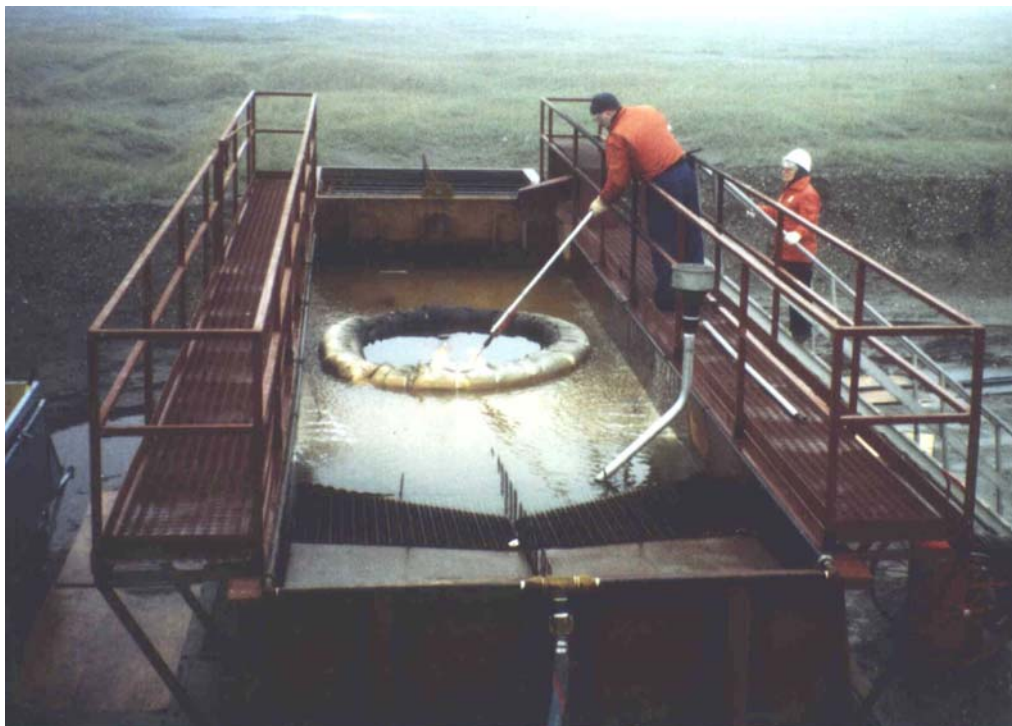
Figure 2 - Burn ring (circle of SWEPI boom) in tank.
