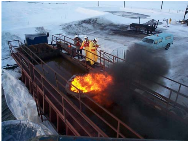
Figure 4-16: Test burn on frazil, or slush, ice.
