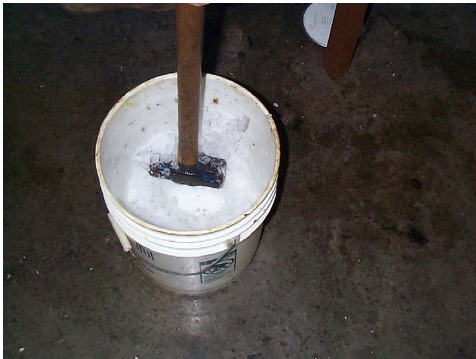
Figure 3-4: Crushing ice cubes used to simulate frazil, or slush, ice.
