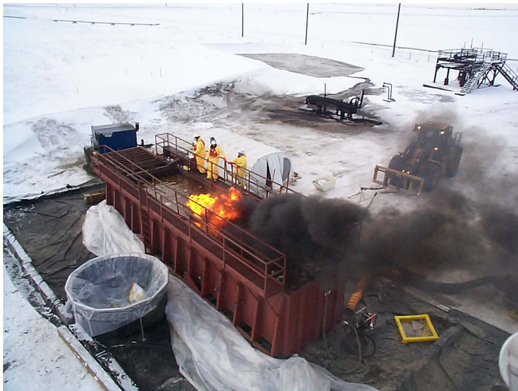
Figure 4-2: View of test burn in tank from lift basket.
