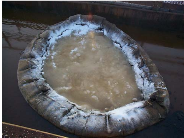
Figure 4-15: Fresh frazil, or slush, ice in ring prior to adding oil.
