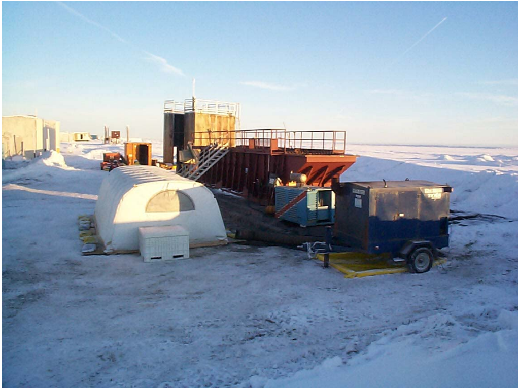
Figure 4-1: Transportable wave tank at the Fire Training Ground.
