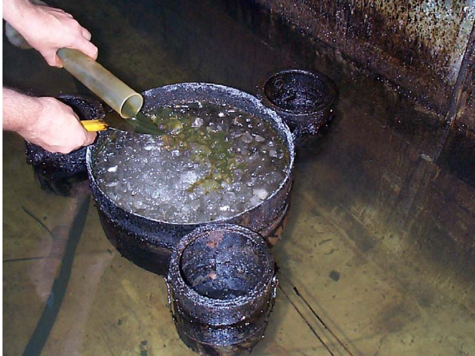
Figure 3-7: Adding Northstar crude to test ring.
