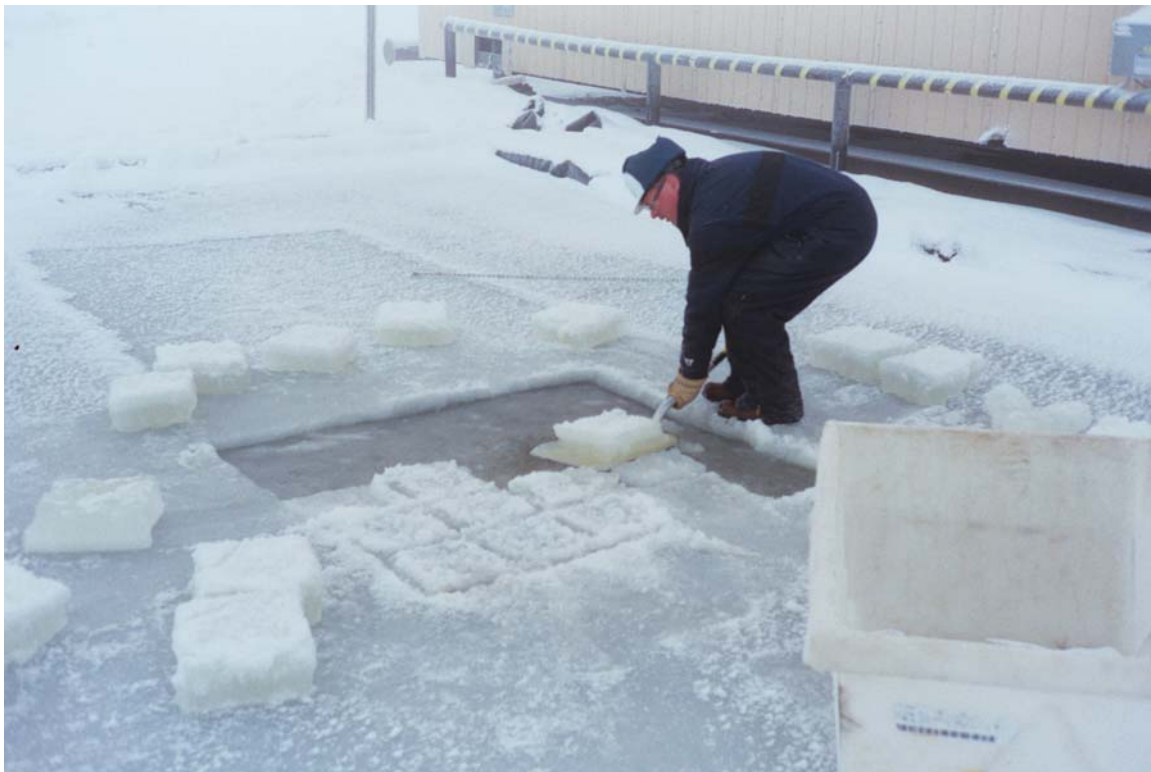
Figure 4.2-1: Removing 30 cm “brash” ice blocks from the test sheet.
