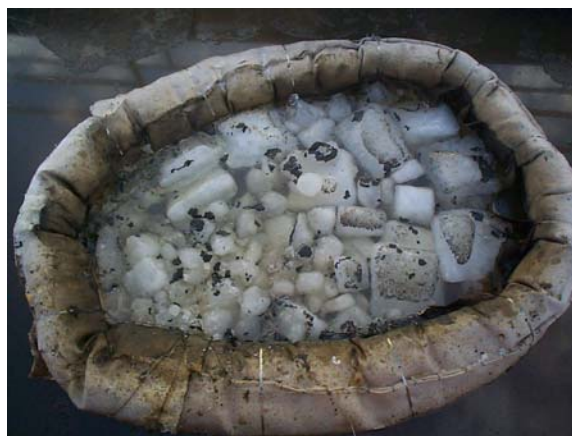
Figure 4-14: Brash ice after burn and residue recovery.
