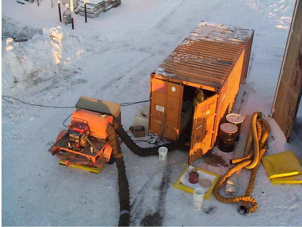
Figure 4-10: Container used for oil storage, measurements and gelled gas igniter preparation.
