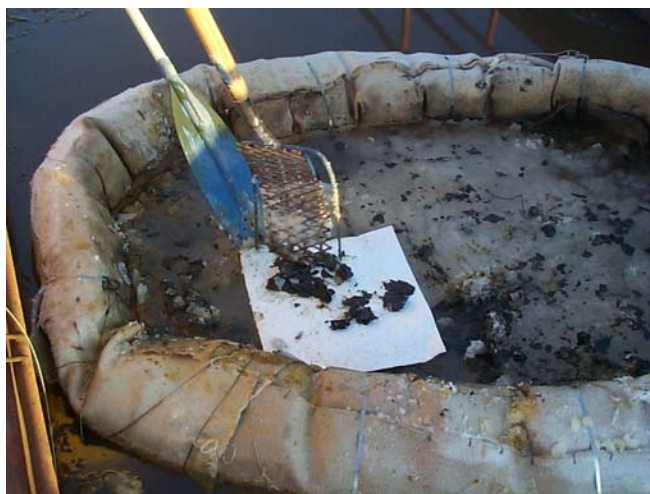
Figure 4-17: Recovering residue from burn ring after burn on frazil, or slush, ice.
