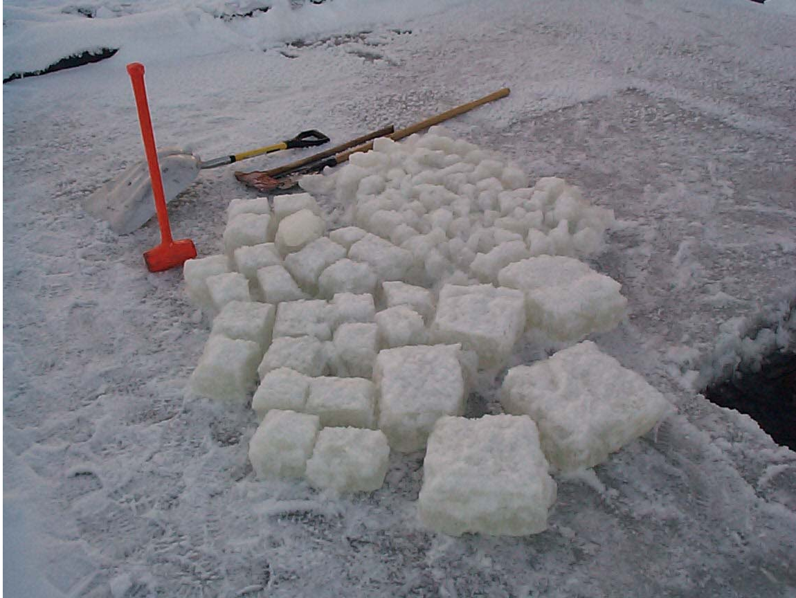
Figure 4.2-2: Final distribution of brash ice piece sizes prior to loading into burn ring.
