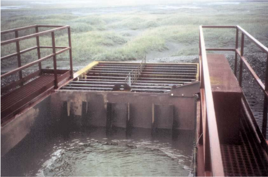
Figure 4-3: Wave board and back-wave absorber panels.
