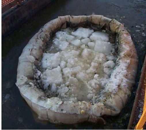
Figure 4-12: Brash ice in ring prior to oil addition.
