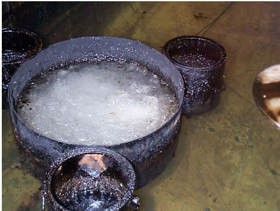
Figure 3-6: Crushed ice in test ring prior to oil addition.
